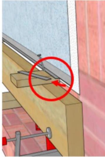
Figure 33 - Cutout of the rail (coating support part) – exterior view
