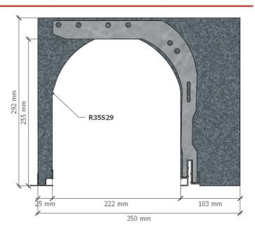
Option brackets and ligatures [PDF]: in accordance with the technical advice of the CSTB, the reinforced boxes will be ligatures to the chain and fixed to the upper crosspiece using brackets. Brackets and ligatures are available in packs of 500 pieces or integrated into the box during production. Corner option [PDF]: the rails 28FR allow the addition of the sealing and fixing corner with the joinery. These 40x30 mm notched corners are available in packs of 100 pieces or inserted in the box.
