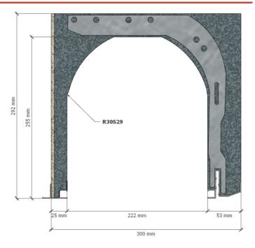
Option brackets and ligatures [PDF]: in accordance with the technical advice of the CSTB, the reinforced boxes will be ligatures to the chain and fixed to the upper crosspiece using brackets. Brackets and ligatures are available in packs of 500 pieces or integrated into the box during production. **Corner option [PDF]**: the rails 30FR allow the addition of the sealing and fixing corner with the joinery. These 40x30 mm notched corners are available in packs of 100 pieces or inserted in the box.
